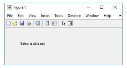
• Specify the text that appears in the component by setting the component String property to the desired text, in this case Select a data set.
