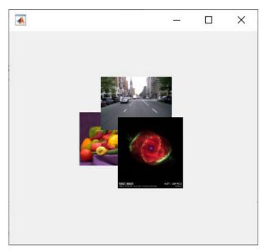
To modify the stacking order in your app, use the **uistack** function. For example, bring the image of the street to the top by rearranging the stacking order of the images.
