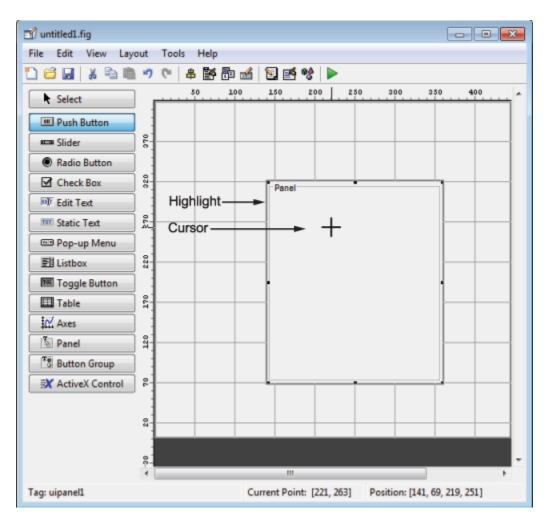
Assign a unique identifier to each component in your panel or button group by setting the value of its Tag property. See "Assign an Identifier to Each Component" on page 18-8 for more information.
