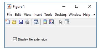
• Specify the check box label by setting the String property to the desired label, in this case, Display file extension.
