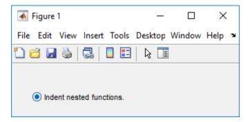
• Specify the radio button label by setting the String property to the desired label, in this case, Indent nested functions.
